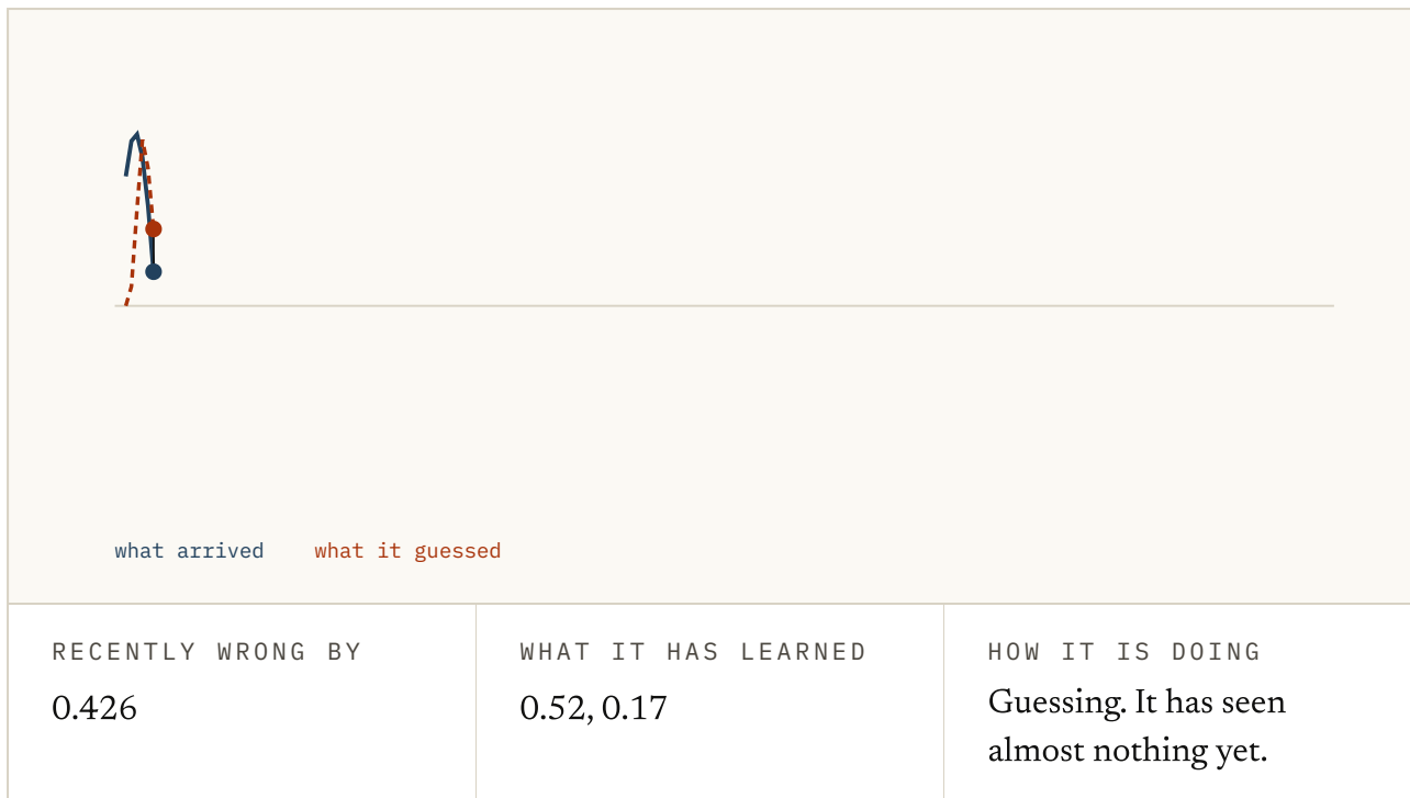
FIG. 3.3 Press Run. The predictor guesses the next number from the previous two, and is corrected a little after every guess. It starts at zero and knows nothing. Watch the dashed line climb onto the solid one, then look under What it has learned: two numbers that nobody supplied, reached by being wrong and adjusting.
